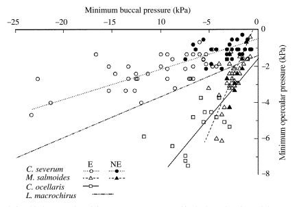
Fig. 3. Relationship between the minimum pressures generated in the buccal cavity and those in the opercular cavity for four predator species in strikes on elusive and non-elusive prey. The lines depict estimates (reduced major axis regressions) of the relationship between minimum buccal and opercular pressures. E, elusive prey; NE, non-elusive prey.
