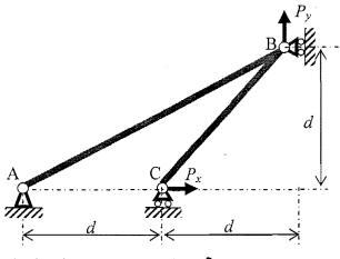
c. Find the stiffness matrix for the structure. UR PE
