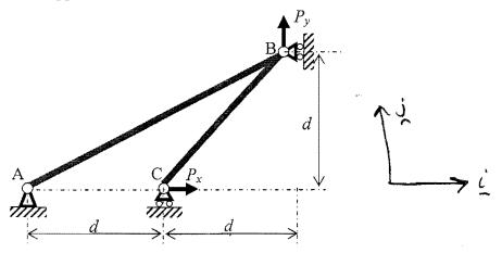
a. Is this truss statically determinate, indeterminate, or a mechanism? Why?
