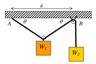
a. Draw a free body diagrams or weight  $W_1$  and  $W_2$  and derive an expression for the angle  $\theta$  as a function of the ratio  $W_1/W_2$ .
