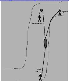
An idealization is shown below. A weight  $W_I$  is suspended by a cable, which is attached to a counter weight  $W_2$  as shown. The pulley at B is frictionless. The goal of this problem is to determine the angle  $\theta$  between the cable and the ceiling when the configuration is in equilibrium. The problem is used here to demonstrate the power of the minimum potential energy principal for mechanical systems.
