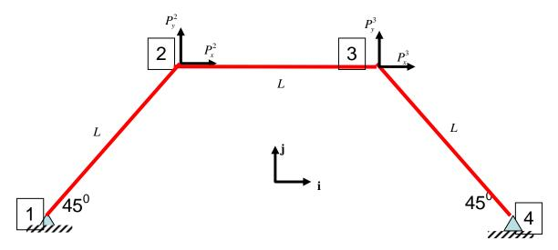
2. Modify the structure above by adding two members as shown below. (Same *EA*) Determine the stiffness matrix for the modified structure.
