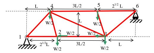
Assume that all the members are made from steel, and have a hollow circular cross-section with OD=2cm and ID=1.8cm. Take L=0.6m and W=700N.
