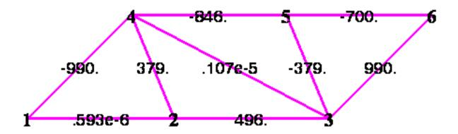
Compressive members of the frame are subject to failure by buckling. Find the buckling load for each compressive member. You might want to use Excel or some such program to find the member lengths and buckling load
