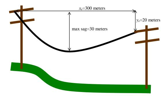
c. The coefficient of linear thermal expansion of the cable in part (b) is  $20\times10^{-6}$  per degrees C. Suppose a cable with length 304 meters at  $10^{\circ}$ C is strung. Find the tension and sag of the cable at  $120^{\circ}$  f ( $50^{\circ}$ C) and at  $-4^{\circ}$  f ( $-20^{\circ}$  C).
