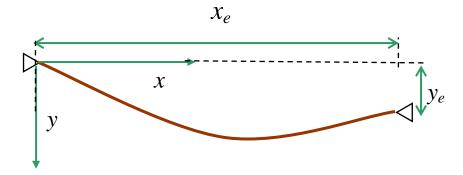
As described in class, the cable will be approximated as a series of N short segments, as shown in the picture below. Each segment has length s=L/N. The shape of the curve will be determined by computing the angle of each segment  $\theta_1, \theta_2 .... \theta_N$  using an EXCEL spreadsheet.
