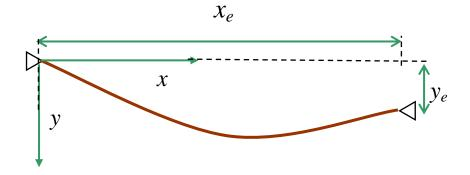
As described in class, the cable will be approximated as a series of N short segments, as shown in the picture below. Each segment has length s=L/N. The shape of the curve will be determined by computing the angle of each segment  $\theta_1, \theta_2....\theta_N$  using an EXCEL spreadsheet.
