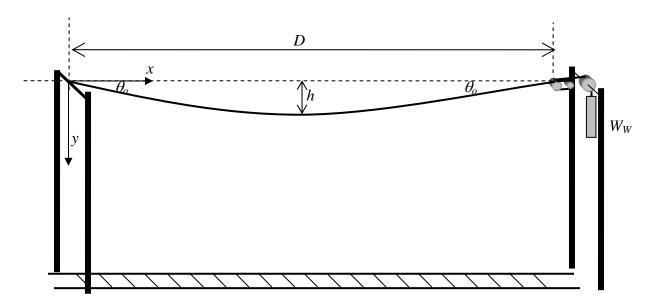
a. Determine the tension  $T_o$  in the electric cable at the endpoints in terms of  $W_w$  and/or  $W_c$ . Neglect the weight of the pulleys and the small segment of cable hanging over the pulley.
