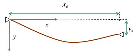
As described in class, the cable will be approximated as a series of N short segments. Each segment has original length  $s = L_O/N$  and weight  $\omega s$ . When deformed, the length of each segment will be  $s_i$  with  $s_i > s$ . The shape of the cable is determined by the angles  $\theta_0, \theta_1, \theta_2, \dots, \theta_{N-1}$  and lengths  $s_0, s_1, s_2, \dots, s_{N-1}$  of each segment.
