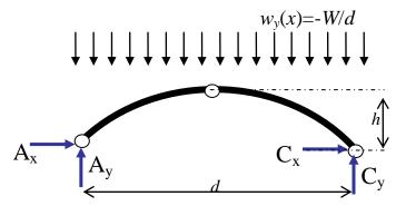
b. Now consider a more refined estimate of the dead loads. The load at the center of the arch is taken to be 57kN/m and extends linearly to the supports, where it has the value of 109kN/m. Determine the reactions due to the bridge weight and plot the internal bending moment, shear, and axial force. Compare the two bending moment distributions. Use symmetry!
