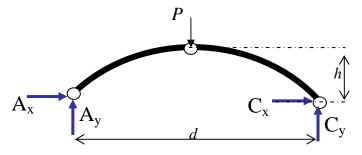
Members AB and BC are two-force members and so the force lines of action pass through AB and BC, respectively. By symmetry, the forces are the same.  $A_y=C_y=R\sin\phi=P/2$ .  $R=P/(2\sin\phi)$ ,  $\phi=\tan^{-1}(h/2d)$   $A_x=-C_x=R\cos\phi=Pd/(4h)$
