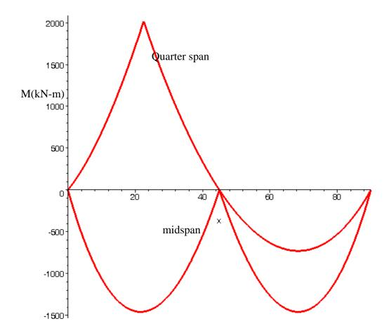
c. Which of these two live load situations gives the highest moment when the 7500kN dead load of the bridge is included? You can use the estimate for the moments due to dead load arrived at in problem 3a of problem set 6.
