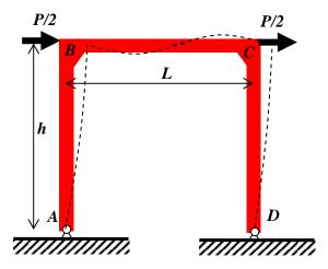
a. To approximately analyze a pinned frame subject to a horizontal load, a hinge is often assumed at the crossbeam midpoint. Find the base reactions as well as the forces and moments transmitted through the joints B, and C, and the forces transmitted through the central hinge. Draw the moment diagram for the members.
