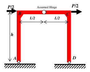
b. Assume full moment connections for this frame, and calculate the deflections and rotations at each joint. Each member has equal properties *EI*. Use the symmetry of the problem, that tells you that the vertical deflection at the hinge must be zero.
