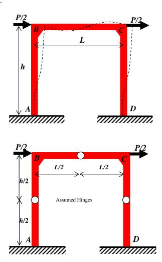
3. In this problem you will find the actual deflections and moments in the frame that is approximated in the previous problem. Assume that the properties EI are the same in the columns and the crossbeam. Neglect axial deformation throughout, so that  $u_x^B = u_x^C$  and  $u_y^B = u_y^C = 0$  and assume full moment connections at B and C.
