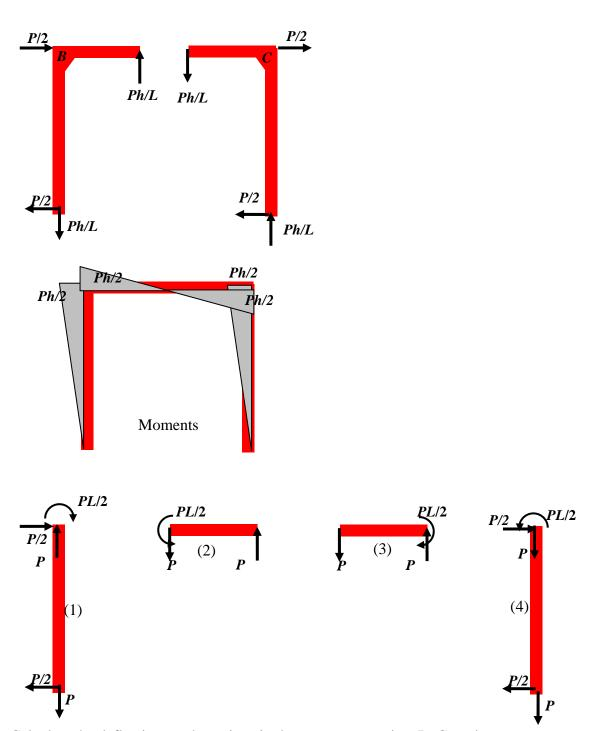
b. Calculate the deflections and rotations in the structure at points B, C, and at the central hinge. You can neglect deflections due to axial loads—include only deflections due to bending. The members have identical values of EI, and let h=L.
