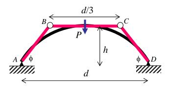
Assume all members of the approximating truss have identical properties E, I, and A, and calculate the deflection under the load.
