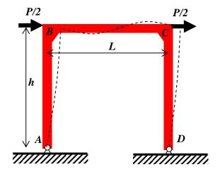
a. To approximately analyze a pinned frame subject to a horizontal load, a hinge is often assumed at the crossbeam midpoint. Find the base reactions as well as the forces and moments transmitted through the joints B, and C, and the forces transmitted through the central hinge. Draw the moment diagram for the members.
