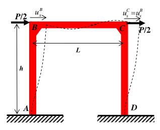
In the figure below, the forces and moments transmitted through joints B and C are shown, along with rotations and displacements of the joints. Note that  $\sum \mathbf{F} = \mathbf{0}$  for the cross beam implies  $B_x = C_x$  and  $B_y = C_y$ .
