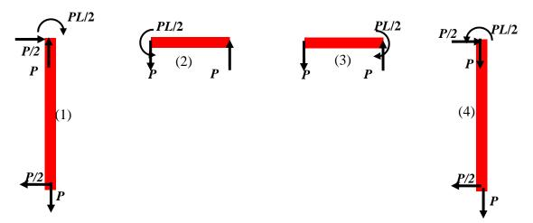
Beam 1: Rotation at A is  $\theta_A = \theta_1^A + \frac{PL^2}{6EI}$ , where  $\theta_1^A$  is the rigid rotation of the member at the base. The second term comes from the beam theory result for a simply supported member with a concentrated moment PL/2 acting on one end. There are no displacements at joint A.
