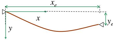
Given cable weight density  $\omega$  and length  $L_0$
