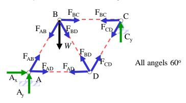
**8 Unknowns**: Force in each member (5):  $F_{AB}$ ,  $F_{BC}$ ,  $F_{AD}$ ,  $F_{CD}$ ,  $F_{BD}$  reaction forces (3)  $A_x$ ,  $A_y$ ,  $C_y$
