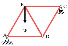
Method of Joints Net force at each joint is zero.
