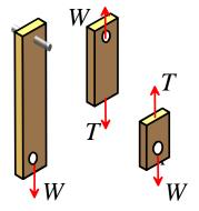
The internal force in a straight 2-force member consists of a force acting normal to the surface of internal surfaces that are perpendicular to the member. Force can be positive or negative. Positive force is tension, negative force is compression.
