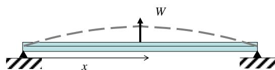
To do the calculation for case II, we must allow the beam to elongate (or no vertical deflection can occur):
