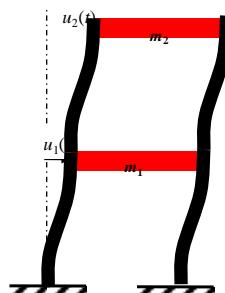
$$\begin{pmatrix} 2k/m - \omega_n^2 & -k/m \\ -k/m & k/m - \omega_n^2 \end{pmatrix} \begin{pmatrix} A_1 \\ A_2 \end{pmatrix} = \begin{pmatrix} 0 \\ 0 \end{pmatrix}$$
