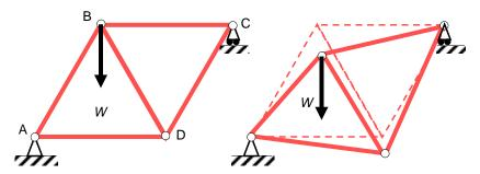
Find the values of the joint displacements for which the potential energy of the structure and its applied loads is a minimum.
