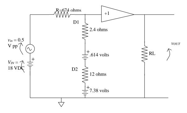
2.) To find the optimal collector current, one has to begin by computing the impedance of the shaker. The reactance of the coil at 60 Hz is 22.6 ohms. The phase angle is
