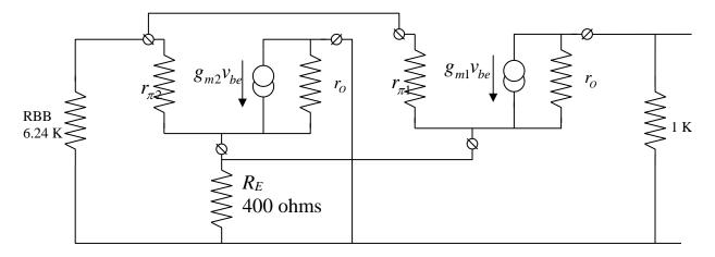
8) The base-emitter voltage is 0.741 volts for 1.0 mA collector current. The base current is 10 uA and the voltage at the node where RB ties to the other two resistors is 2.5 - 1e3\*1.01e-3 = 1.49 volts. Ohm's law gives RB = (1.49 - .741)/1e-5 = 74.9 K.
