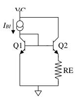
RE. For that reason, its collector and base currents will be less than those of Q1 and so we can very likely neglect at least the base current of Q1.
