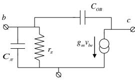
$C_{OB}$  is the capacitance of a reverse biased junction and often has the dependence on voltage of an abrupt-junction. For at least one value of collector-base voltage, it is straightforwardly shown on any datasheet. Often is is given as a graph against VCE.
