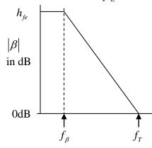
current gain of the transistor. In class, we showed that because of the base-emitter capacitance, the current gain becomes frequency dependent. For a grounded-collector circuit, the gain becomes
