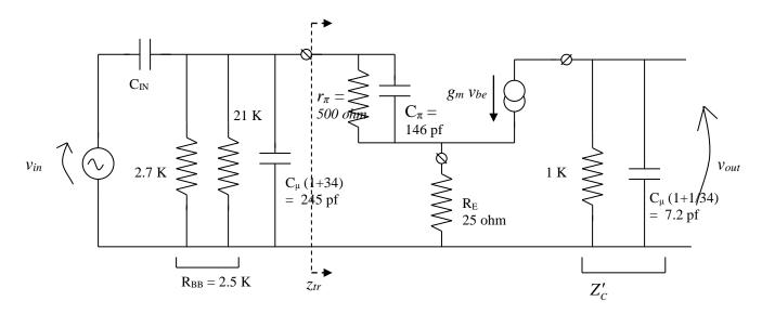
For  $Z_{in}$  we have (neglecting  $C_{IN}$  because it provides only a low-frequency, high-pass cutoff):
