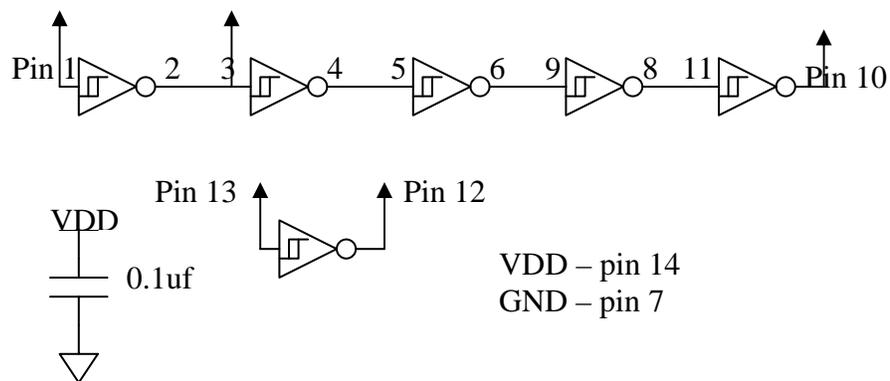
**Prewired SN74LVC04A Connections: The bypass capacitor is on the socket and arrowheads mark available wires for your connections.**
