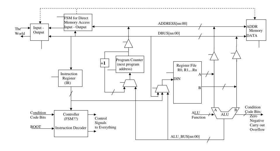
**Simple RTM System with Program Control - aka "***A Computer*": This is most of LabD and its design is my variations on a theme by ARM. The short lines on the sides of almost all the functional blocks are the control lines for that block. For example, the short line just above the DIN bus on the left side of the register file is the set of lines that select what registers feed the A and B buses,
