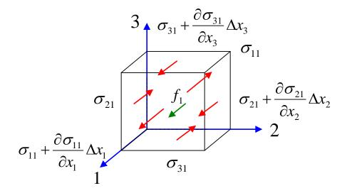
Summing up all the forces in  $x_1$  direction and applying Newton's law,
