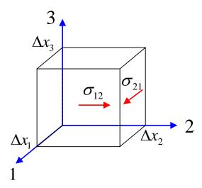
A simpler demonstration of symmetry of stress tensor:
