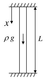
We have shown in the beginning of the semester that the exact solution is:  $u = \frac{\rho g}{2E} x(L-x)$ . Now we discuss how to solve the same problem by using the principle of minimum potential energy.
