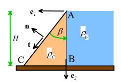
6.1 Write down formulas for unit vectors  $\mathbf{t}$ ,  $\mathbf{n}$  tangent and normal to the back face of the dam, in terms of  $\beta$  (you will need this information for part 6.2 and 6.3)
