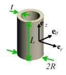
Recall that the stresses in a thin-walled pressurized tube are related to the internal pressure by  $\sigma_{zz} = pR/(2t)$ ,  $\sigma_{\theta\theta} = pR/t$   $\sigma_{rr} \approx 0$
