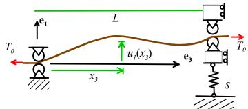
5.1 Write down the boundary condition for the transverse displacement  $u_1$  of the cable at  $x_3 = 0$ .
