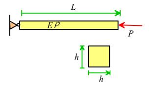
1.2 A beam with h=1cm, L=1m, E=210GPa,  $\rho=1000 \ kg.m^{-3}$  subjected to an axial load P=200N has a natural frequency of 100 Hz. If *h* and *L* are both doubled, and *P* is increased by a factor of 4, what is the new natural frequency?
