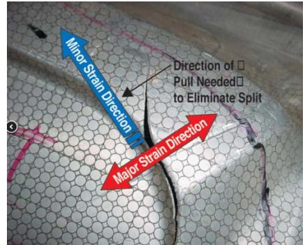
2. ‘[Circle Grid Analysis](#)’ is used to estimate strains induced in sheet metal parts during stamping or drawing. The figure shows a typical example. Suppose that the three lengths  $L_1, L_2, L_3$  on a circle with initial radius  $R$  are measured.
