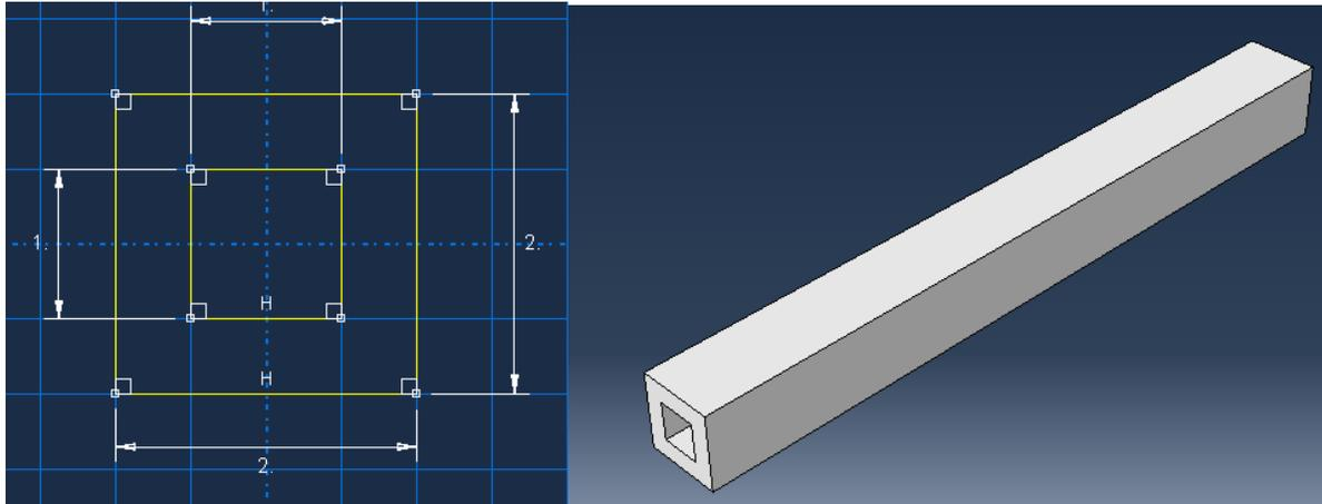
5.2 Next, create a planar 'Discrete Rigid' flat planar part with dimensions 1.5x1.5mm and center at the origin.
