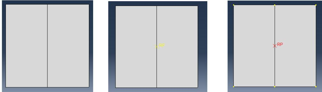
5.4 Assign an isotropic elastic material with Young's modulus  $E=210000$  (units are MPa) and Poissons ratio  $\nu = 0.3$  to the beam.
