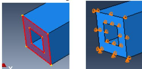
5.9 You can now load the beam by applying forces and displacements to the reference point on the rigid surface part. The reference point is a special type of node, and so also has rotational degrees of freedom; and allows you to prescribe moments. As a first test, apply a twisting rotation  $UR_3 = 0.5$  radians to the reference point on the rigid surface.
