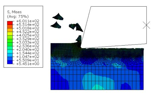
**6. Orthogonal machining model:** In this problem you will set up a simple 2D model of an orthogonal machining process (see the figure). The problem uses several advanced techniques in FEA:
