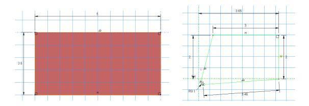
For mesh generation and adaptive meshing we will have to partition the workpiece as shown below. To do this, first partition the block down the middle – select the 'partition by shortest distance between two points'
