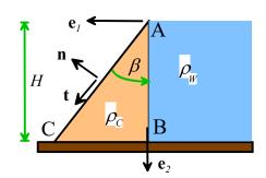
6.1 Write down formulas for unit vectors  $\mathbf{t}$ ,  $\mathbf{n}$  tangent and normal to the back face of the dam, in terms of  $\boldsymbol{\beta}$  (you will need this information for part 6.2 and 6.3)
