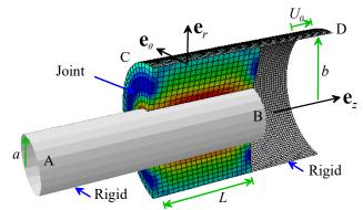
The goal of this problem is to estimate the axial force necessary to produce displace the shaft CD, and hence determine the stiffness of the joint.
