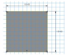
enter density in N milliseconds<sup>2</sup>/mm<sup>4</sup>, which makes  $\rho = 10 \times 10^{-3}$  in our chosen unit system (note that wave speeds in m/s and mm/millisecond are identical). Assign the part a homogeneous section with these properties.
