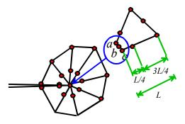
connected together, and (ii) the mid-side nodes 2 and 7 are moved to the quarter-point location on the element side. This magically produces the necessary singularity in the strain.
