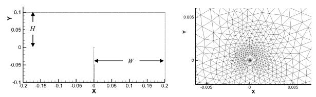
You can find a finite element mesh for this problem in the file called crack\_tri6.in. The mesh contains two regions: elements 1 to 1246 are regular 6 noded triangles, and mesh the region outside r=0.0006. Elements 1247-1256 are crack tip elements, which lie inside a circular domain with radius 0.0006 units. You can thus evaluate the domain J integral over the circular region of crack tip elements using
