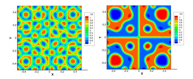
1. The Cahn-Hilliard equation is one of the most famous equations in materials science, and is an example of a more general description of materials with evolving structure known as 'phase field' models. The original purpose of the Cahn-Hilliard equation was to describe spinodal decomposition of a single-phase liquid or solid into two phases, but it has since been extended to model many other phenomena.
