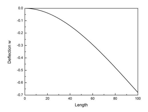
The rotation angle of the beam is -0.0102 at L=100. While for the analytical solution,  $\Phi = \frac{FL^2}{2EI}$
