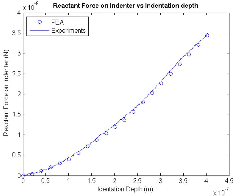
Figure 8 Reactant force acting on the indenter versus the indentation depth for new material parameters found for 8-chain model.
