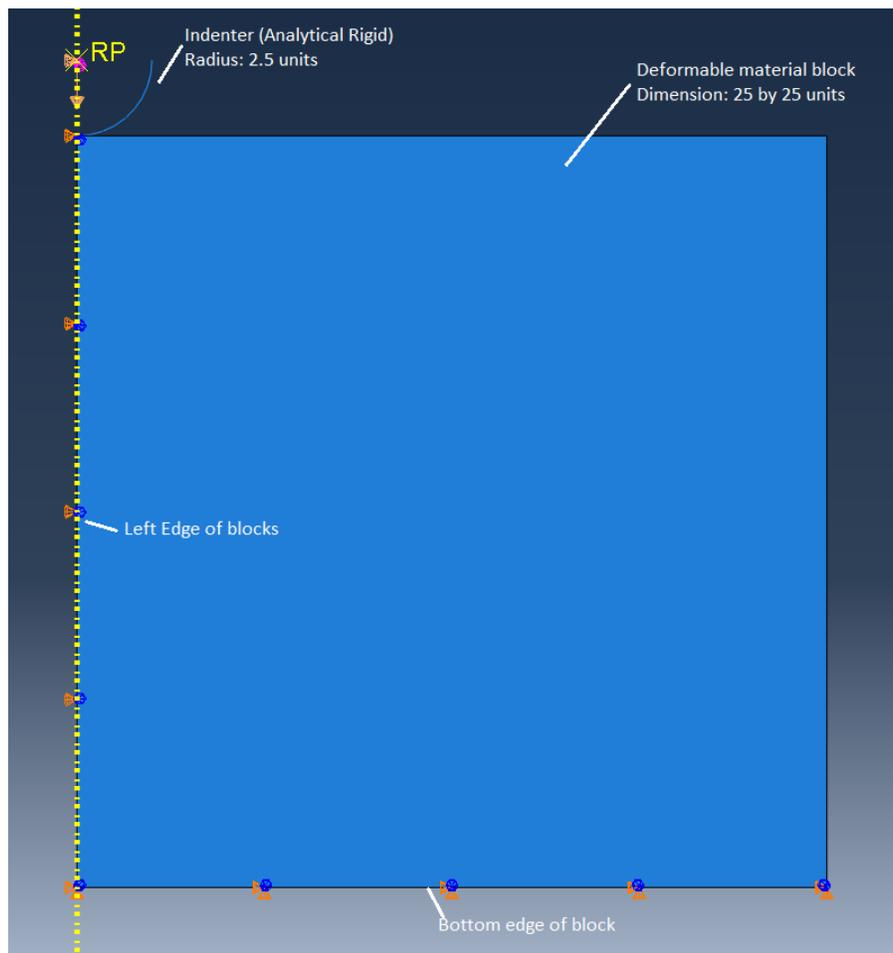
Figure 1 The basic geometry and assembly of model in abaqus.
