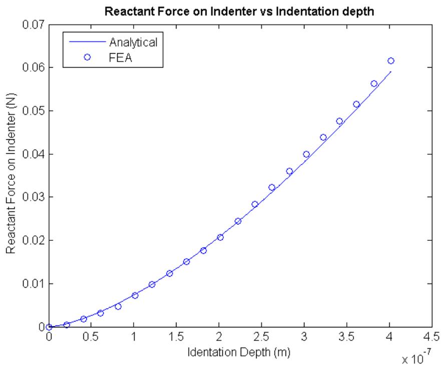
Figure 5 Reactant force acting on indenter versus the indentation depth for a linear-isotropic material
