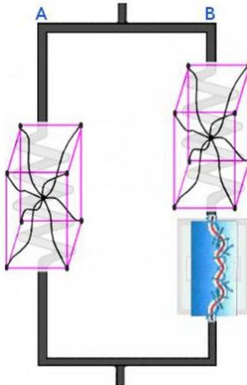
Figure 6 Rheological representation of Bergstrom-Boyce model (Source: <http://polymerfem.com/content.php?77-bergstrom-boyce-model>)
