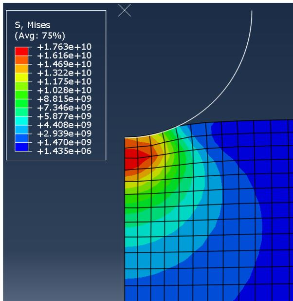
Figure 4 Close-up of von-mises stress produced in the material block modeled as linear-isotropic material. (Note that the units of von-mises stress are in  $\text{kg}/\mu\text{m}.\text{s}^2$ )
