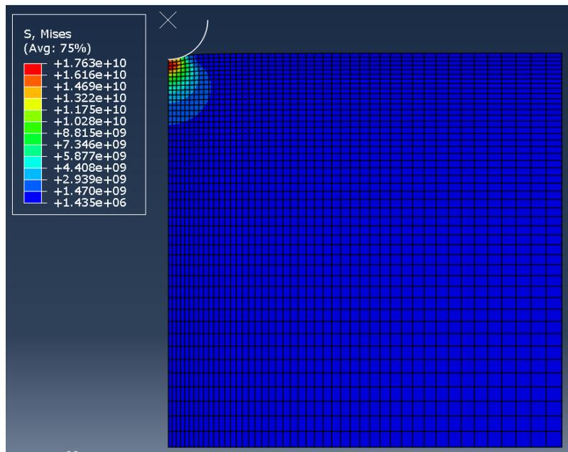
Figure 3 Von-mises stress produced in the material block modeled as linear-isotropic material. (Note that the units of von-mises stress are in  $\text{kg}/\mu\text{m}.\text{s}^2$ )
