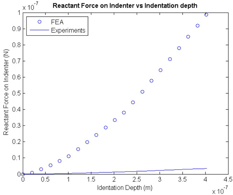
Figure 7 Reactant force on indenter vs the indentation depth for material following 8-chain model with parameters borrowed from BB-model.
