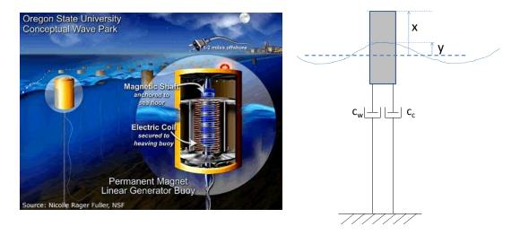
The picture shows a magnetic shaft surrounded by an electric coil. The shaft is attached to a cable fixed to the ocean bottom, while the coil is attached to the buoy. As the buoy bobs up and down due to the ocean waves, the coil passes back and forth across the magnetic shaft and generates an electric current (you will learn about this in EN 52). That current is captured by various electronics and sent back to shore. Thus, mechanical energy in the wave is converted into electrical energy.
