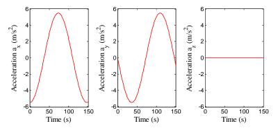
6.1 Let  $\mathbf{r}=\mathbf{R}\mathbf{i}$  and  $\mathbf{v}=\mathbf{V}\mathbf{j}$  denote the position and velocity vectors of the aircraft at time t=0. Find formulas for the position, velocity and acceleration vectors of the aircraft in terms of *R*, *V* and *t*.
