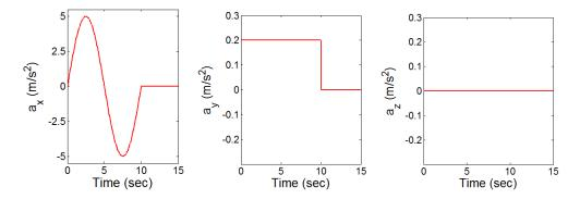
**1.** A <u>three-axis accelerometer</u> mounted on an <u>inertial platform</u> with fixed orientation measures three components of acceleration shown in the figure (the first figure can be approximated as a sinusoidal function). If the platform is initially at rest at the origin, what is its position vector after 15sec?
