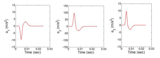
7.5 Suppose that a helmet starts at rest and has orientation  $\theta = 0$ . An impact is then detected with acceleration signals shown in the figure (note that  $a_3(t) = -a_1(t)$ ). If the mass of the head is 4.5kg, what is the peak impact force? What is the angle  $\phi$  of the impact location on the head?
