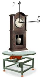
$\sum F_{Y} = -mg + T\cos\theta = m\ddot{Y}$  and  $\sum F_{Z} = T\sin\theta\sin\Omega t - N\cos\Omega t = m\ddot{Z}$ , show that the equation of motion is reduced to  $\ddot{\theta} + (g/l)\sin\theta - \Omega^{2}\cos\theta\sin\theta = 0$ . Here *T* is the tension and *N* the force normal to (x, y) plane, transmitted through the pendulum bar.
