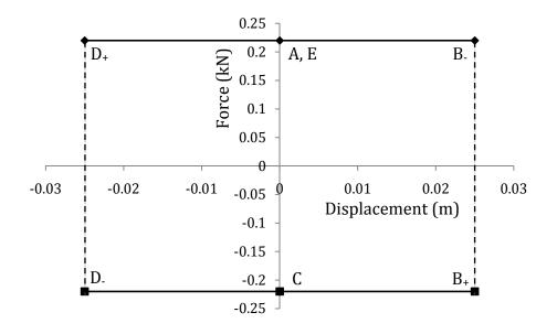
Work dissipated =  $0.22(kN) \times 0.025(m) \times 4 = 0.022(kJ)$  [2 points]
