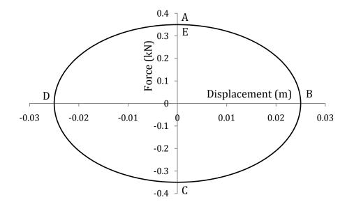
Work dissipated =  $0.35(kN) \times 0.025(m) \times \pi = 0.027(kJ)$  [2 points]
