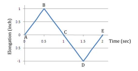
(1.1) Draw the force - displacement diagram for the force applied to the spring during the displacement cycle. Mark the corresponding points of A, B, C, D and E on the drawing. What is the work dissipated during this cycle?
