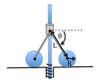
In the mechanism shown, each of the two wheels (mass=m<sub>w</sub>, radius=R) is connected to a collar via a slender bar (length=L, mass=m<sub>b</sub>). The collar slides (mass=m<sub>c</sub>) frictionlessly on a vertical shaft, and hits a spring (spring constant=k) when the bars are in a horizontal configuration. The wheels roll without slipping.
