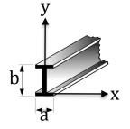
For top/bottom beam (both the same):  $a = a, c = L, m = \rho t a L$ distance from CG = L/2  $I_G = \frac{1}{12}m(a^2 + L^2) + mL^2/4 = \frac{m}{12}(a^2 + 4L^2)$  $I_G = \frac{\rho t a L}{12}(a^2 + 4L^2)$
