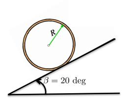
Consider a ring of radius mass M and radius R, initially released from rest on an incline of 20 degrees. The coefficient of kinetic friction is  $\mu_k$ , and the coefficient of static friction is  $\mu_s$ .
