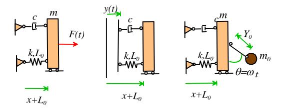
**3.** The specifications for a force plate designed for jump performance analysis can be found at this website. A force-plate is essentially a spring-mass system – the force acting on the plate is determined by measuring the change in length of the spring x (the spring actually a piezoelectric transducer). The force is then estimated by multiplying the length change by the spring stiffness kx. This works perfectly for a static force, but if the force applied to the plate varies with time, then
