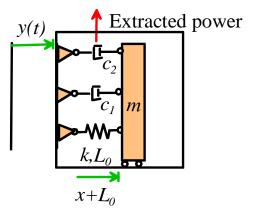
$$\frac{1}{\omega_n^2} \frac{d^2 x}{dt^2} + \frac{2(\zeta_1 + \zeta_2)}{\omega_n} \frac{dx}{dt} + x = -\frac{K}{\omega_n^2} \frac{d^2 y}{dt^2}$$
