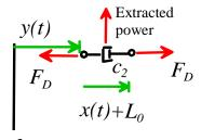
4.4 Hence, show that instantaneous power generated is  $P(t) = c_2 X_0^2 \omega^2 \cos^2(\omega t + \phi)$
