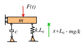
$kx(t) \neq F(t)$ . The goal of this problem is to work out how to design the system to minimize the error in measuring a dynamic force, and to calculate the maximum frequency of a fluctuating force that can be measured accurately. Suppose that:
