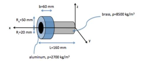
1.1. Determine the mass moment of inertia about the x-axis. 1.2. Determine the mass moment of inertia about the y-axis.
