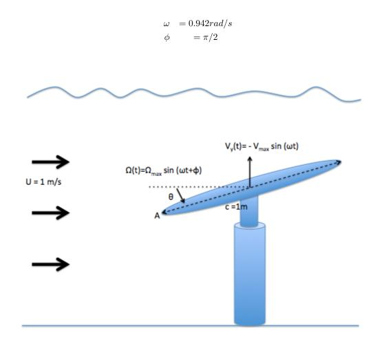
3.1. Plot the position of the leading edge, A, as a function of time.
