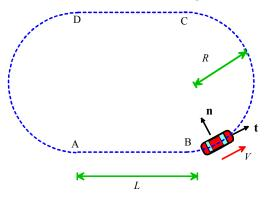
5.1 Assume the vehicle travels at constant speed from B to C, and hence write down a formula for the acceleration vector in  $\mathbf{n}$ , t coordinates in terms of speed and R. Hence find a formula for the shortest time to travel from B to C.
