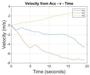
(iii) Estimate the velocity by differentiating the position vector, and plot this estimate as a function of time. You can do this by calculating the change in position between two successive readings, and dividing by the time difference between them, e.g. if x(i) denotes the *i*th value of *x*, then
