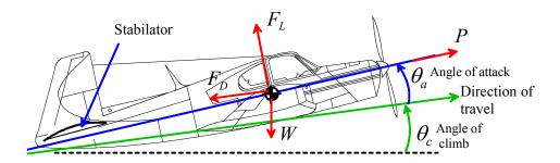
The aircraft has wing area  $A_W$  and flies at (variable) speed V. It is subjected to four forces:
