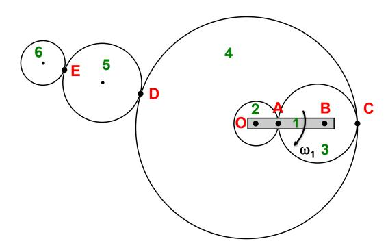
a) [1 pt] What is the gear ratio  $\omega_4/\omega_6$ ?
