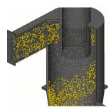
Suppose the air contains a distribution of spherical particles, with radius b and mass density  $\rho$ . As a rough approximation, we can represent the effect of the spiraling airflow as a rotating rigid bar that exerts a normal reaction
