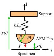
The tip is subjected to: (i) a force from the spring; (ii) an attractive surface force F (acting downwards on the tip), which is related to x by  $F = F_0 \frac{x}{d} \exp(-x/d)$ ; and (iii) a drag force resisting motion of the tip
