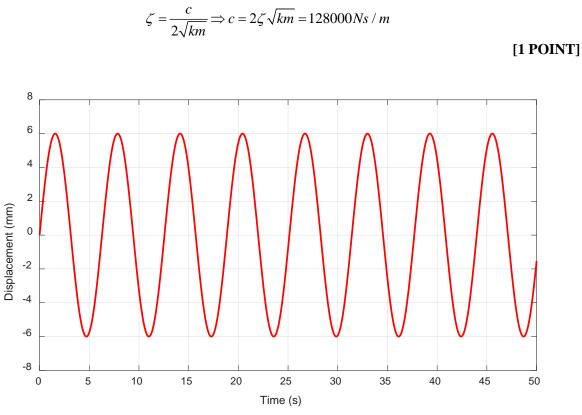
4.2 The figure shows the measured displacement of the system during operation. The blades have a radius of 40m, and the total mass of the system  $(m + m_0)$  is 25000kg. Assuming that the rotor can be balanced by adding mass to the tip of one blade, estimate the mass that must be added to balance the rotor.
