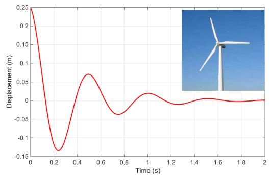
**4** An unbalanced wind-turbine is idealized as a rotor-excited springmass system as shown in the figure. The mass *m* represents the tower, and  $m_0$  represents the combined mass of the three rotor blades. The spring and damper represent the stiffness and energy dissipation in the tower. The rotor is 'unbalanced' because its center of mass is a small distance  $Y_0$  away from the axle. The total mass  $(m + m_0)$  of the system is 25000kg.
