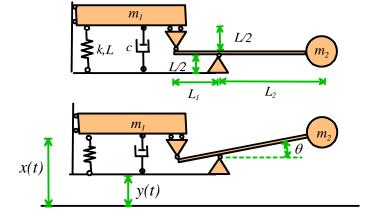
3.1 Draw free body diagrams showing the forces acting on the mass  $m_1$  and the pendulum assembly (see the figure).
