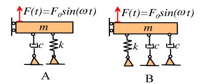
The formula for amplitude is  $X_0 = KM(\omega / \omega_n, \zeta)F_0$ . When  $\omega = \omega_n$  the magnification  $M = 1/(2\zeta)$  where  $\zeta = 2c/(2\sqrt{km})$ . Removing a dashpot does not change the undamped natural frequency and halves  $\zeta$ . The amplitude will double.
