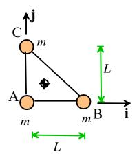
6.2 Calculate the 2D mass moment of inertia of the system about the center of mass
