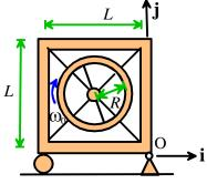
4.1 Find formulas for the mass moments of inertia of the frame and the wheel (about the center of the wheel).
