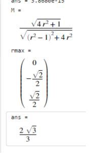
This shows that the biggest vibrations will occur when  $\omega = \omega_n / \sqrt{2} = 22.2rad / s$ The vibration amplitude is  $X_0 = Y_0 M_{\text{max}} = 2Y_0 / \sqrt{3} = 1.15mm$
