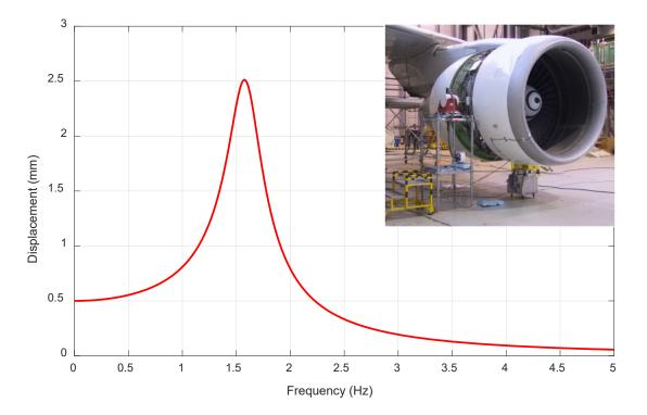
**4** As part of the airworthiness certification process, the rotating parts of a jet engine are prevented from turning, and the engine is subjected to an external horizontal harmonic force  $F(t) = F_0 \sin \omega t$  with amplitude  $F_0 = 250$ N. The amplitude  $X_0$  of the steady-state horizontal vibration  $x(t) = X_0 \sin(\omega t + \phi)$  of the engine is measured.
