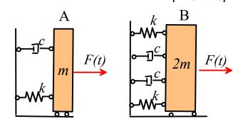
Where  $k_{eff}$  is the effective stiffness. The two springs in B are in parallel, so the effective stiffness of B is twice that of A. This implies that the amplitude of B will be half that of A, i.e. 0.5mm.
