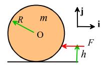
2.1 Draw a free body diagram showing all the forces acting on the ball (include gravity and assume no slip at the contact)
