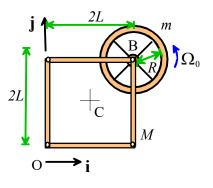
4.1 Find formulas for the out-of-plane components of the mass moments of inertia ( $I_{Gzz}$ ) of the frame (about its center of mass at C) and the wheel (about the center of the wheel), in terms of *m*, *M*, *R* and *L*.
